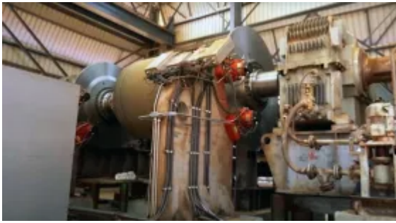
Fig. 16: Tail drive pulley with brake a caliper arrangement
