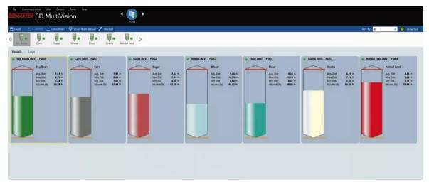
This example shows how the user can view multiple silos on a single screen, getting an overview of inventory for their operation.
