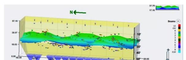
In this screen image, the topography of material is displayed and used to detect level per section.
