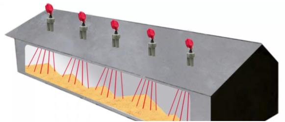
Several 3DLevelScanners are strategically mounted on the roof with each scanner measuring multiple points in a 70-degree beam angle.
