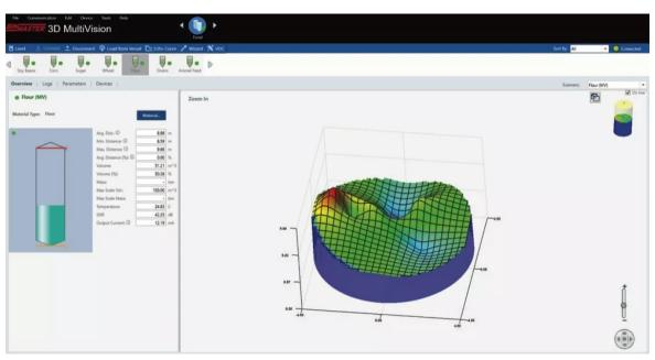
Upon selecting a single tank, the user can get specific details about minimum, maximum, and average volume and view the 3D visual.
