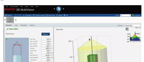
It is evident from the 3D graphic that material is disbursed evenly and the cone is up. The average, minimum, and maximum levels are displayed along with the volume and mass.
