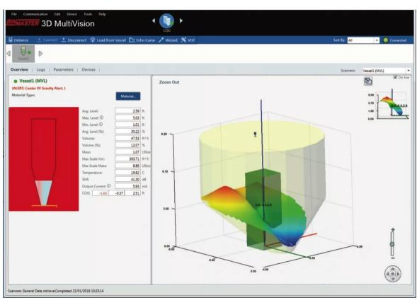
Alert status: the 3D visual indicates that as the vessel has been emptied, material has built up on one side of the vessel.
