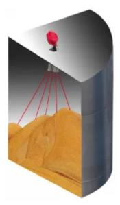
This illustration shows material piled unevenly in a silo segment and how the 3DLevelScanner measures mul-tiple distances across the material surface to account for irregularities when calculating volume.
