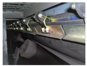
Conveyor skirting maintains a dust seal between the chute structure and the conveyor belt. (Pictures: @Dyna Engineering)
