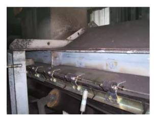
DYNA Engineering's Flexiseal® low maintenance conveyor skirting does not require any adjustments.
