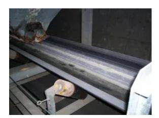
Belt mistracking due to material spillage and lack of conveyor skirting.
