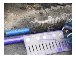
The prototype (top) compared with the new CFC cleaner (bottom). The finger elements can be easily replaced during operation.
