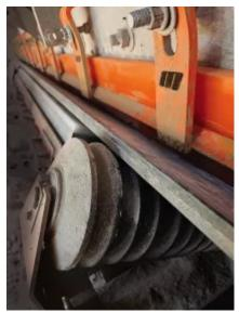
The Martin<sup>®</sup> Urethane Skirting seals the transfer chute enclosure to prevent dust and spillage.
