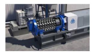
The polysius® booster mill is available in four sizes from 300 to 1800 kW installed power. (Picture: ©thyssenkrupp Polysius GmbH)
