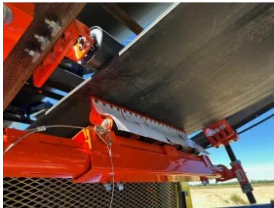
The mounting assembly firmly secures the secondary cleaner to the stringer.
