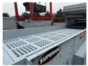
Superior's new HD scalping screen handles a maximum feed size of 18-inches (457mm). (Picture: ©Superior Industries, Inc.)
