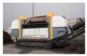
The UNTHA XR3000C mobil-e shreds scrap tyres down to a fraction size of approx. 50 mm and separates metal parts using an over belt magnet
