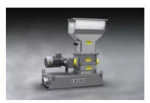
Infeed hopper length is twice that of the feed throat to accommodate conveyor-feeding of irregular shapes and sizes of hard, soft and/or fibrous materials.
