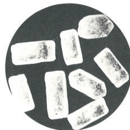
Dull, scratched and dust-coated crystals shown here are from a conventional dryer.
