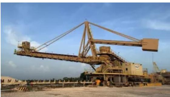
TAKRAF's 6,000 t/h rail-mounted stacker assembled on site and ready for final items prior to being put into operation. (Picture: ©TAKRAF GmbH)
