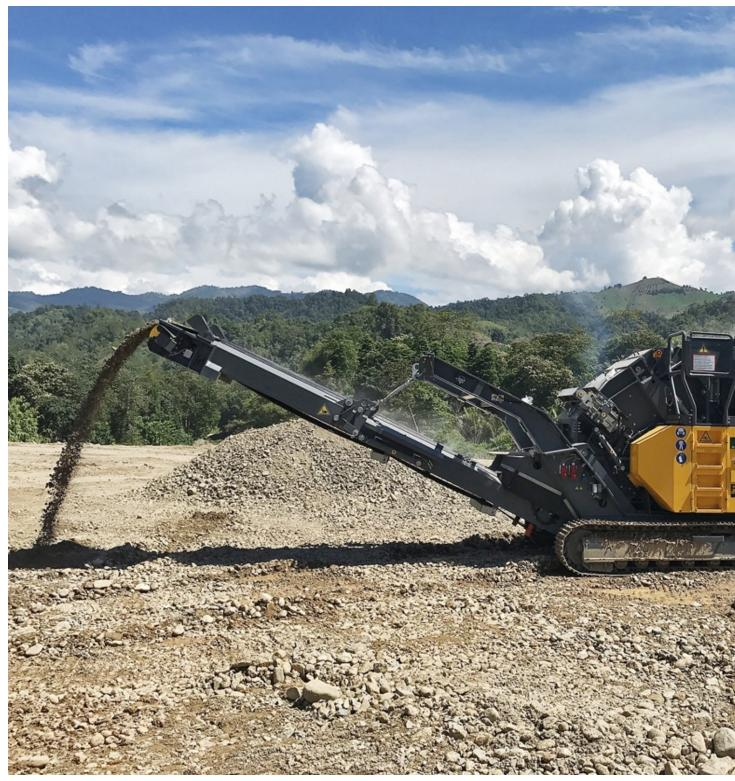
The RM 70GO! 2.0 processes extremely abrasive river basalt in a single pass. The crusher unit replaces the combination of jaw and cone crushers.
