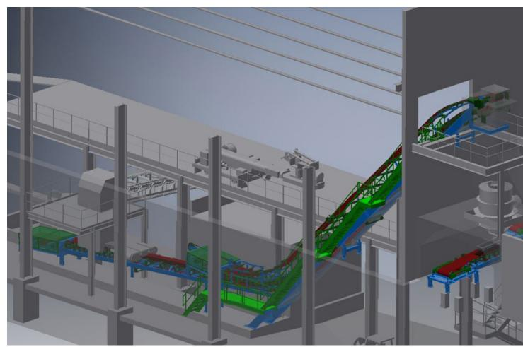
The DSI Sandwich high angle conveyors will serve as transfer conveyors elevating crushed pebble ore, each at a rate of 135 t/h and a 45° incline for Continental Gold's Buriticá project in Antioquia, Columbia.
