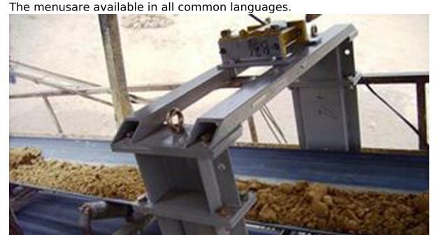
**Customized**On request, we supply the components together with a special mounting frame for installation of the detector and shield. The robust steel frame is optimized in terms of radiation protection and stability and ensures a reliable measurement. By applying the optimal arrangement for different options of sources and detectors we find the best solution for our customers.
