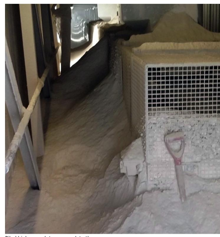
Piled high enough to encapsulate the tail pulley, the dust blocked walkways, posing a potential hazard.
