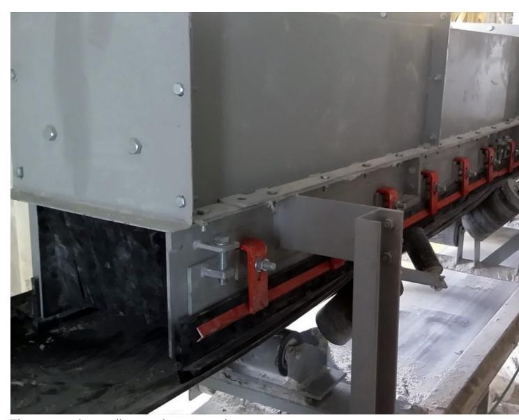
The external wear liner and apron seal help prevent damage to the chute wall.
