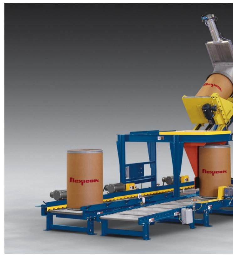
TIP-TITE® Dumping System for drums containing bulk solids allows safe, high-capacity transfer of materials by automatically positioning, dumping and removing of drums in repeated cycles.
