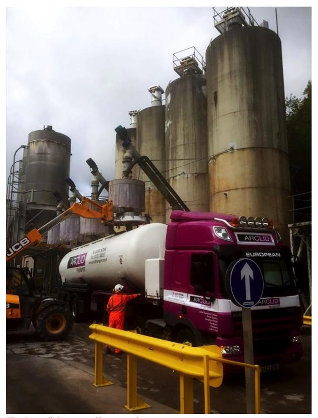
The Russell Compact Sieve used to check-screen marble powder during loading of delivery tankers.
