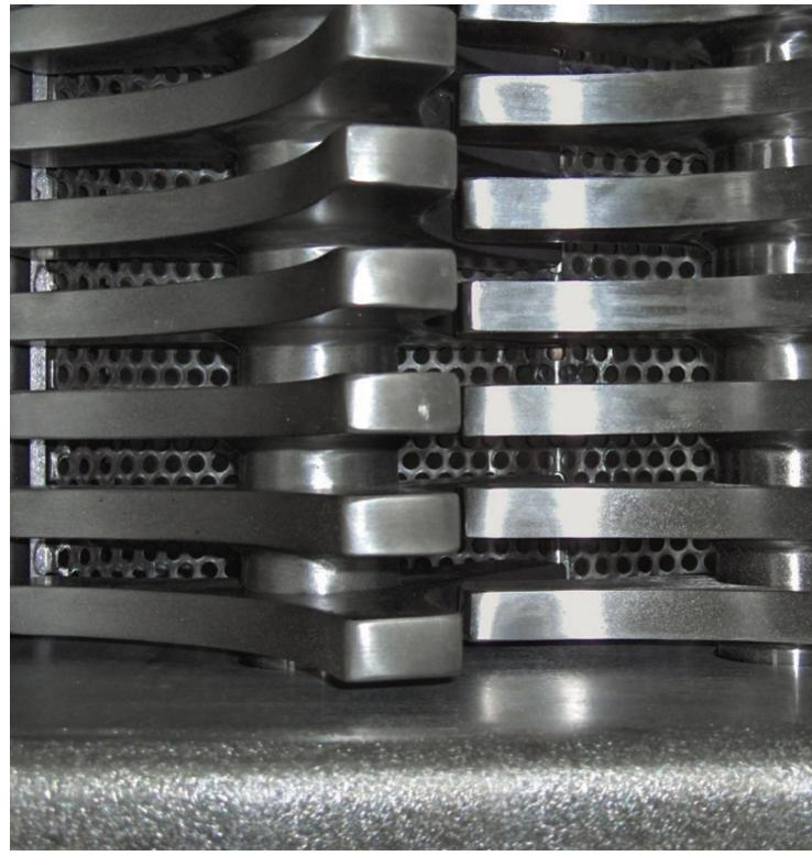
Dual rotors with three-point, singlepiece, abrasion-resistant breaking heads rotate with minimum clearance above a curved, perforated bedscreen with apertures from 25 to 64 mm in diameter.
