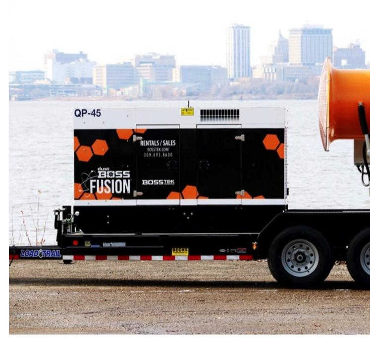
The DB-60 Fusion dust suppressor features a Tier IV Final-compliant generator.
