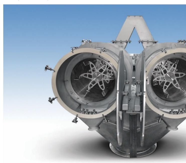
Each screening chamber of the Quick-Clean design features a cantilevered shaft with no end bearing on the hinged end plate, allowing the screen cylinder and paddle assembly to slide freely from the shaft end for rapid screen changes, cleaning and inspection.
