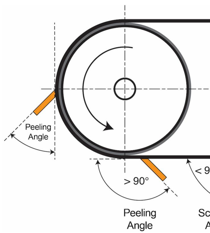
A negative rake angle delivers outstanding cleaning performance with low belt pressure.
