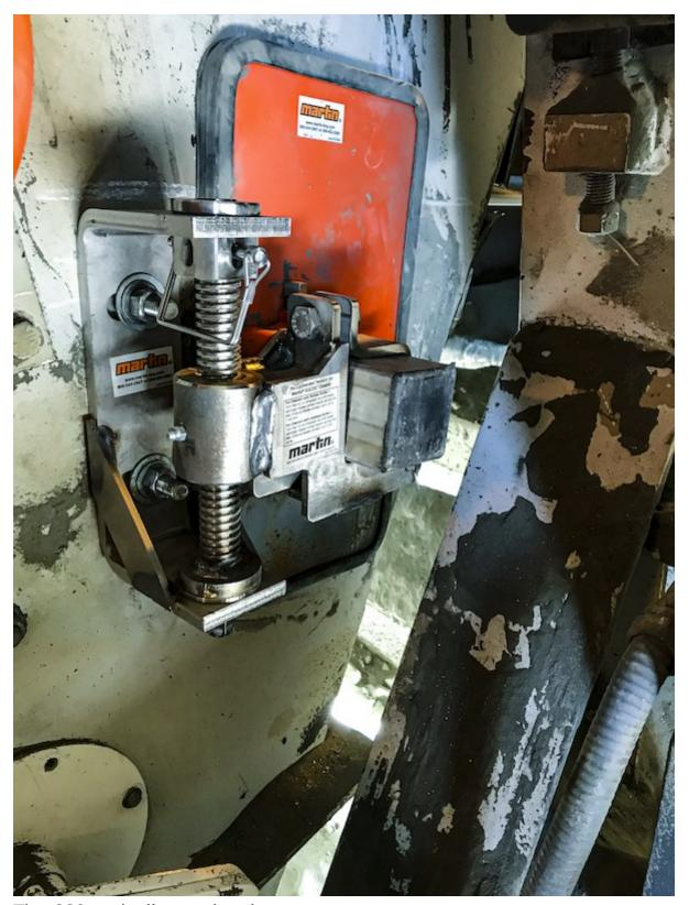
The CS2 typically requires just one retensioning during its lifespan, helping to reduce cost of ownership.
