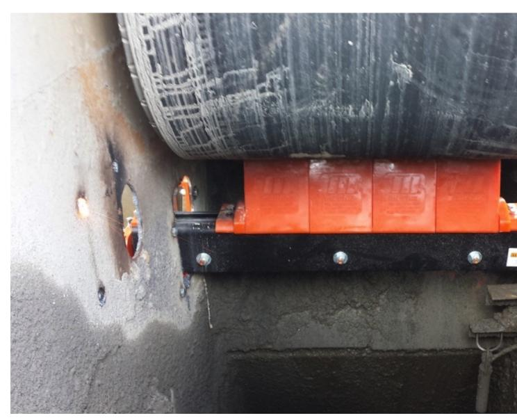
Sixteen additional secondary belt cleaners were attached behind the header, equipped with tungsten tipped blades.
