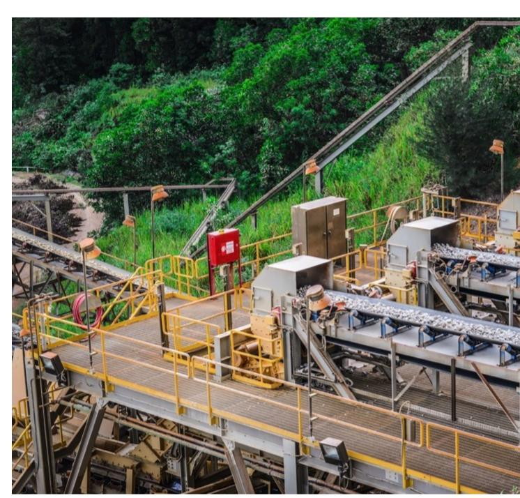
The original conveyor belt cleaners could not manage the overburden, resulting in carryback that caused equipment failures and downtime.
