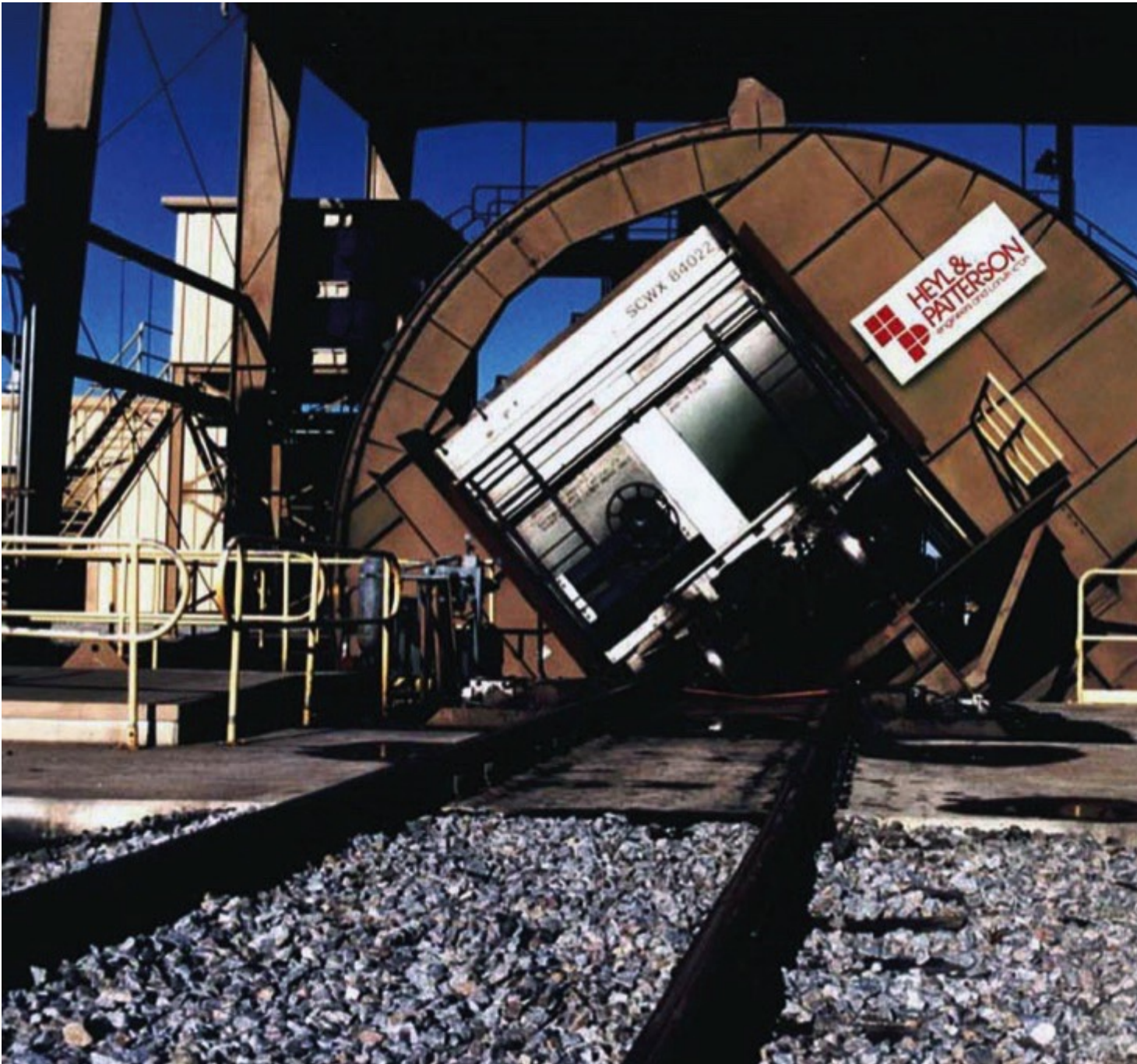
Railcar dumper at work.
