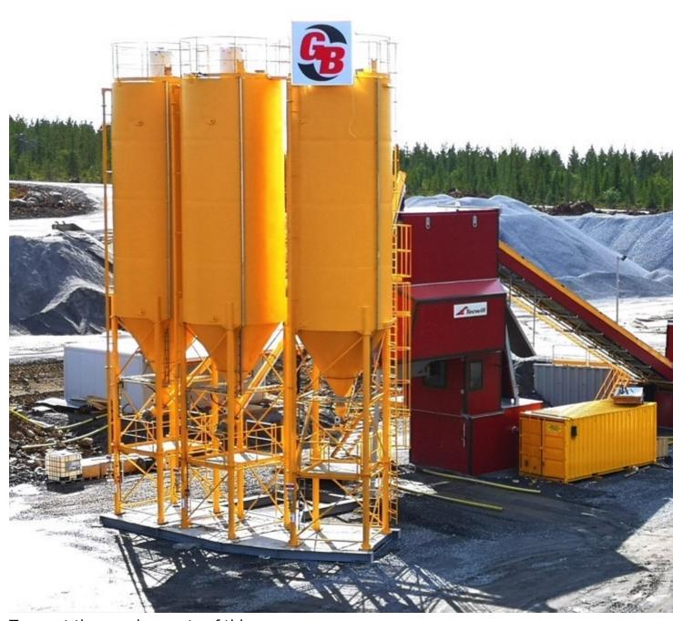
To meet the requirements of this project, Tecwill built a mobile concrete batching plant with a twin-shaft batch mixer at its heart. (Pictures: ©BSH Sonthofen)
