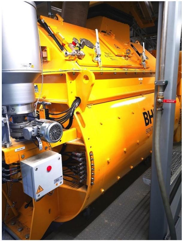
The twin-shaft batch mixer from BHS-Sonthofen is known for its reliability, short mixing times and high homogeneity.
