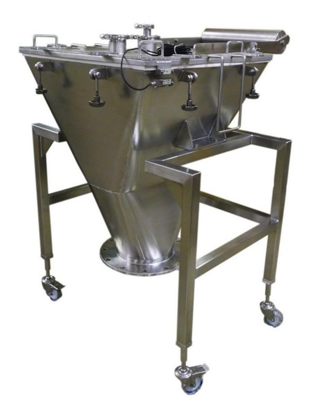
The equipment was fabricated in grade 316 stainless steel with all contact surfaces mirror polished and contact welds made crack and crevice free; the finish promotes flow and discourages any possible build-up of powder. The design was informed by powder testing carried out by Ajax onsite in Ireland. Assessment of the material enabled Ajax to produce a hopper and transition chute that works with the poorly flowing powder as well as effectively interface with the site's existing mill.
