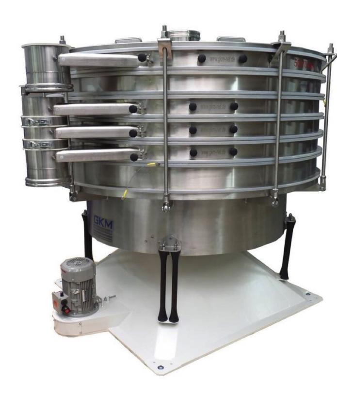
GKM's range of modular Flat Deck Screeners sifts powders and granules gently while obtaining the required particle size without material degradation—which is crucial when sieving more friable products. These modular, multi-deck screeners are designed to remove the oversize product in the top deck. The remaining material passes through the appropriate number of decks for the application, down to the bottom deck, where the very fine product is collected.
