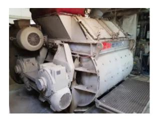
Maximum performance, even during continuous use: The twin-shaft batch mixer blends the complex formula in just 90 seconds.
