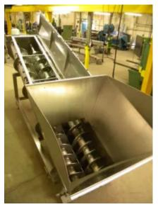
An Ajax twin screw feeder previously supplied to improve throughput, handling and inspection of pork rind at Essentia. (Picture: Ajax
