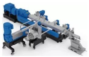
The new ZSK FilCo filtration compounder markedly simplifies recycling of post-consumer recyclate (PCR) and any highly contaminated polymer: Filtration and compounding can now take place in one single production system. (Photo: Coperion, Stuttgart Germany)
