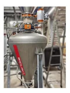
Gericke pneumatic dense phase conveying system for cocoa powder. (Picture: ©Gericke)
