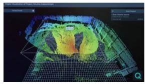
Point cloud of the waste piles in the hall. The Lidar sensor calculates the inventory volume very accurately through a surface scan. (Source: Blickfeld)
