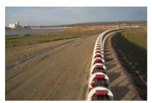
TAKRAF's 1,400 t/h tube conveyor with a length of 4,535 m for ash and gypsum at a power plant in Bulgaria. (Picture: ©TAKRAF GmbH)
