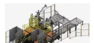
Safety is a top priority in the design of the new bulk bag-filling system. The equipment is fully enclosed with safety fencing and features interlocked access gates to prevent unauthorised access while ensuring that the equipment operates safely and efficiently.
