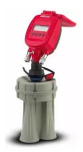
The 3D level sensor measures and maps multiple points on the material surface. Measuring irregular material surfaces ensures improved accuracy when calculating volume. Its accompanying 3DVision software shows a 3D image representing the topography inside the silo. This image indicates buildup that can cause sidewall damage in the silo and cone up or down conditions. MultiVision software allows viewing of multiple silos at a single location.
