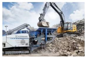
Kleemann MOBIREX MR 130i EVO2 at work with the John Deere excavator 345GLE recycling concrete in California. (Pictures: ©WIRTGEN GROUP)
