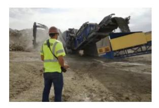
The MR 130i EVO2 can be operated conveniently from a safe distance with the radio remote control.
