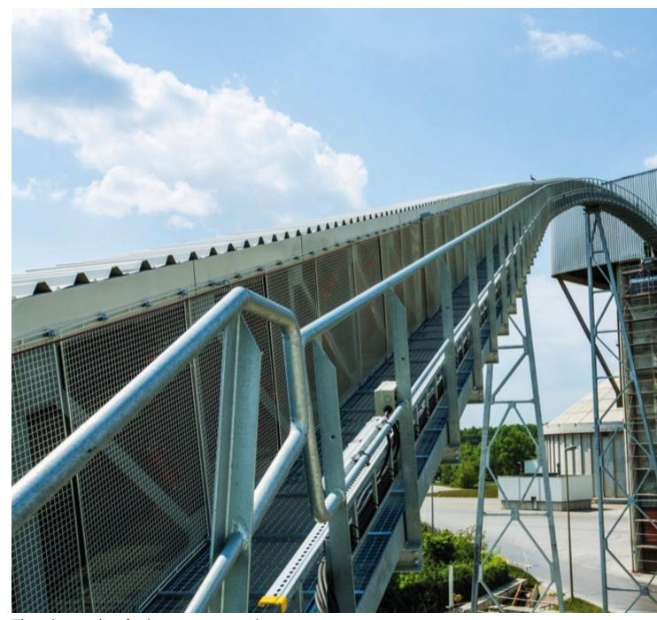
The alternative fuels are conveyed from the storage to the main burner, low in noise and dust-proof. (Picture: ©Beumer Group GmbH & Co. KG)
