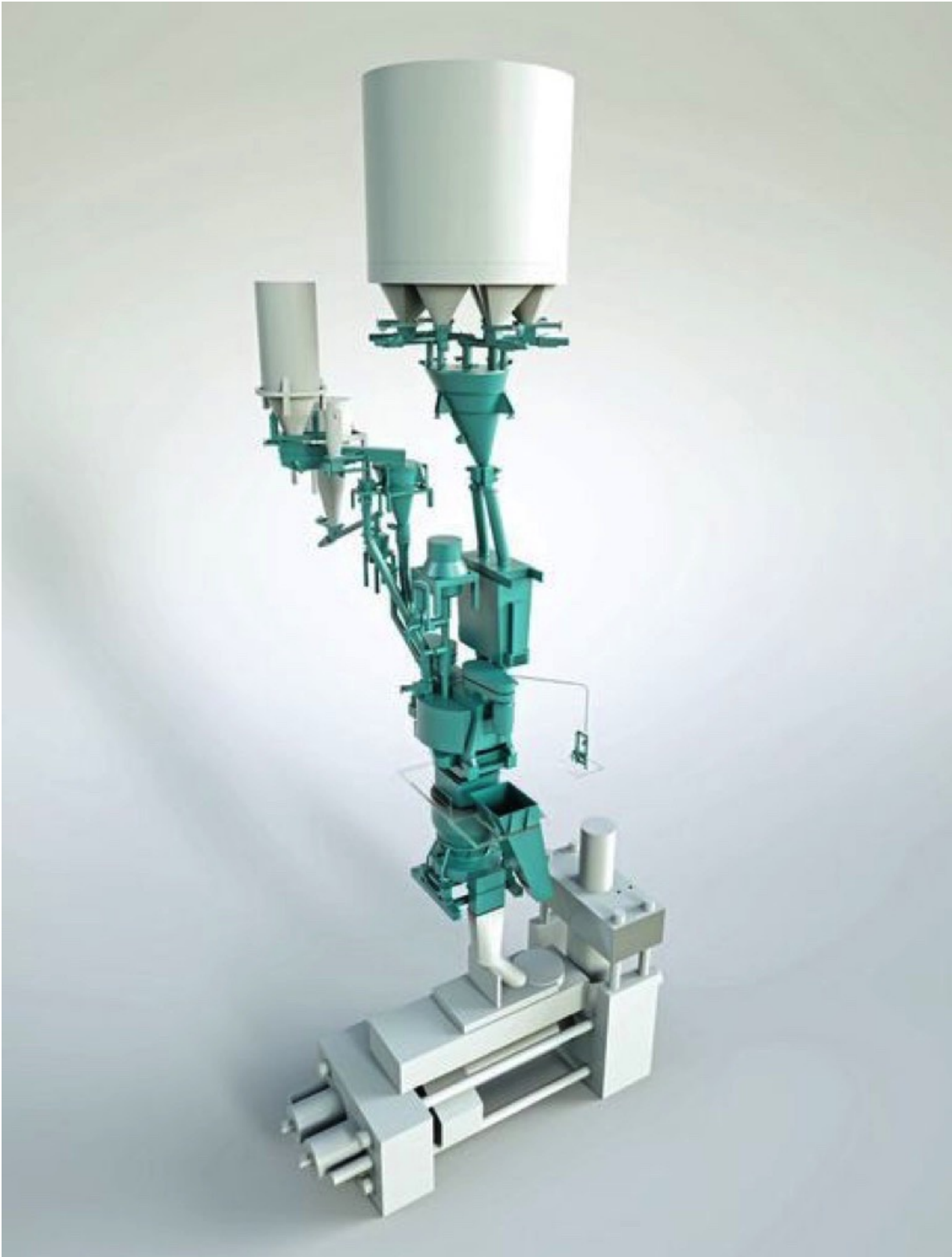
Eirich plant layout for the preparation of graphite electrode compounds. (Picture: @Eirich)
