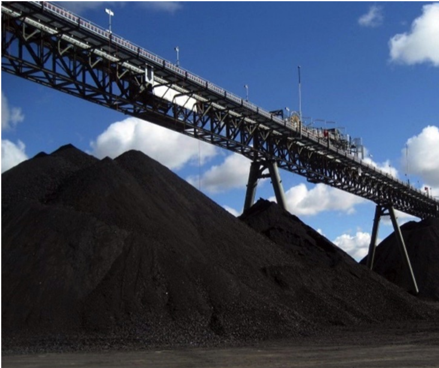
Fig. 1: Coal stockpile with trestle legs supporting the conveyor (Pictures: ©The Authors/TUNRA Bulk Solids)
