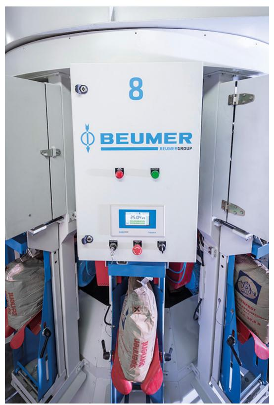
Beumer Groups fillpac® rotating filling machine is equipped with extensive features. (Pictures: © Beumer Group)
