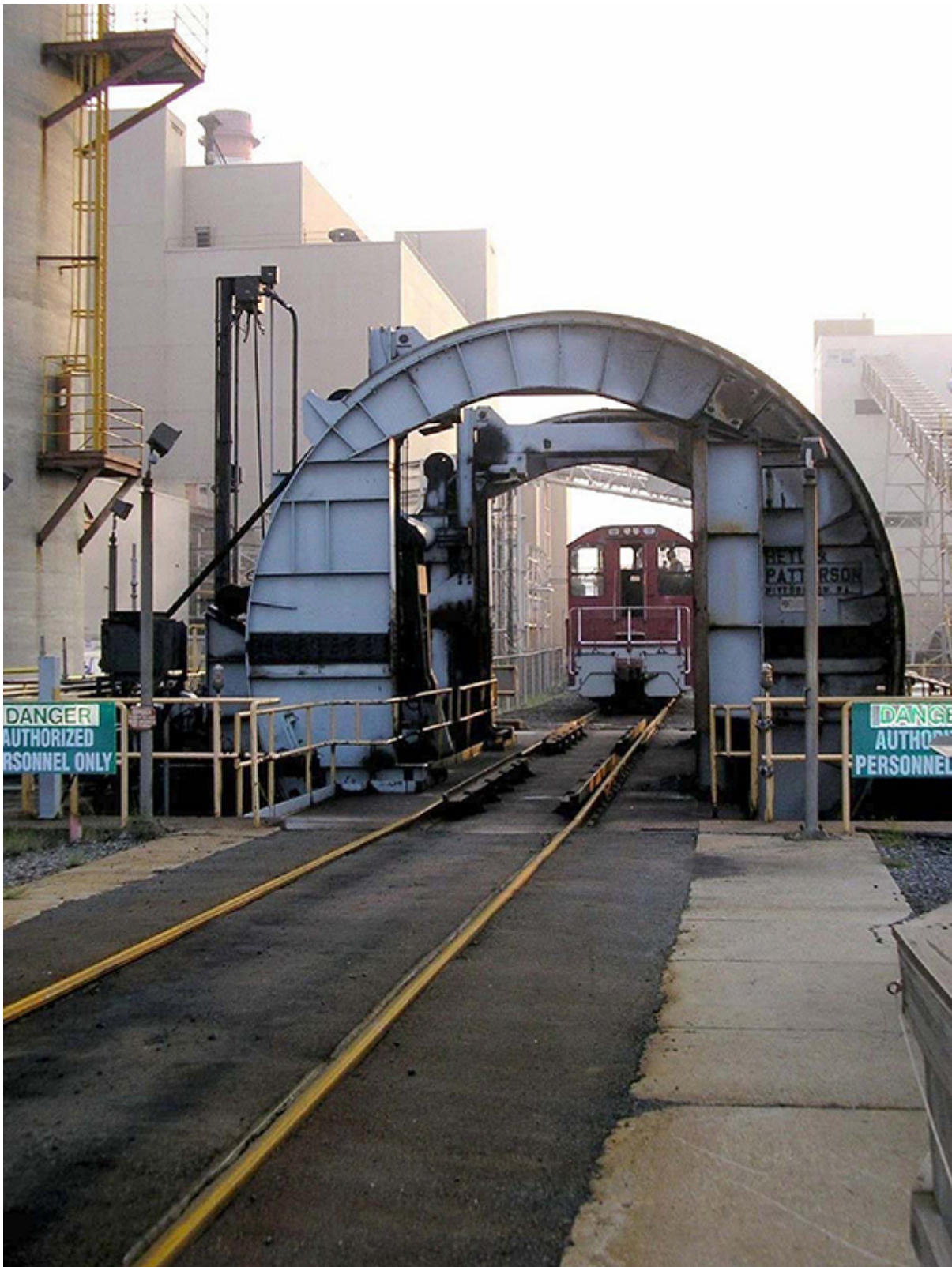
A train is approaching the railcar dumper at an iron ore smelter. (Pictures: © Heyl & Patterson)
