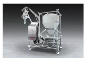
Flexicon's mobile sanitary IBC unloading station can be moved to multiple locations in the facility or rolled to a cleaning station for quick
