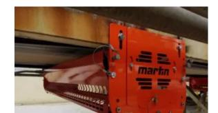
Return roller guards ensure detached rollers don't pose a hazard to workers or harm the system.
