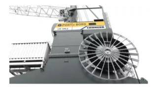
The all-electric LPS 420 E supports a more environmentally friendly infrastructure at the port, able to operate without the need for hydraulic oil or a diesel engine. (Pictures: ©Liebherr-MCCtec Rostock GmbH)
