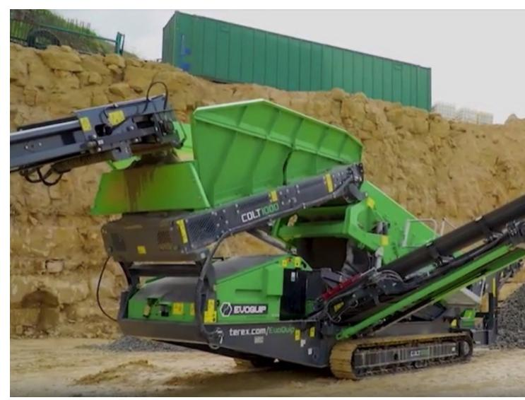
The Colt 1000 achieves excellent conveyor discharge heights and by coupling a broad belt on the fines the machine distinguishes itself from the competition.
