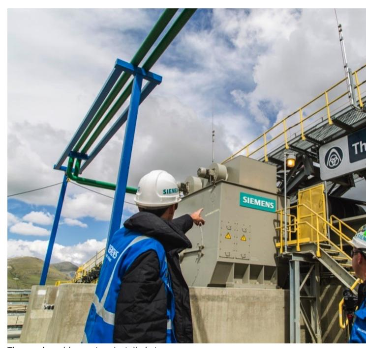
The gearless drive system installed at the Las Bambas Copper Mine includes four low-speed synchronous motors (4.4 MW, 66 rpm) and the associated
