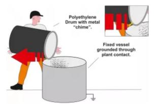
The situation in the plastic processing plant, when the powder cloud ignited.
