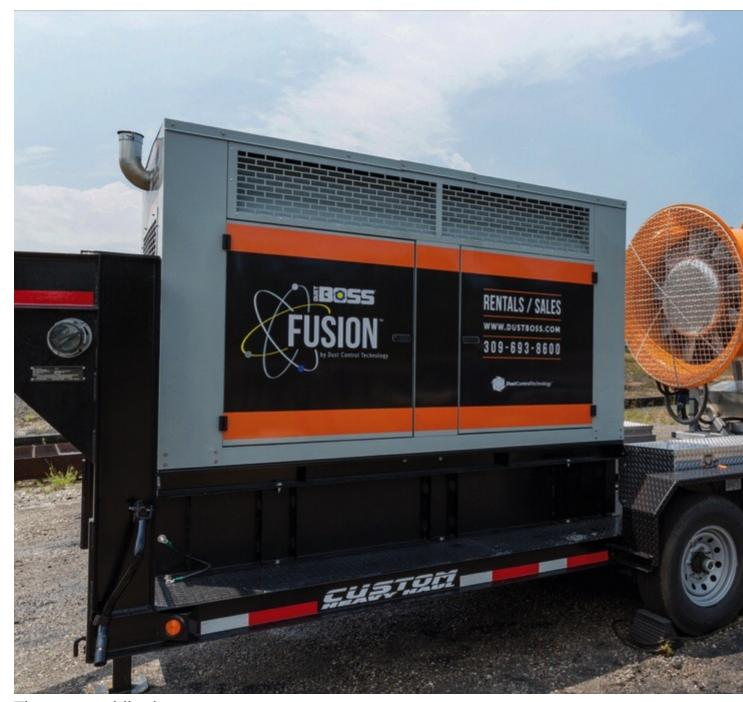
The new mobile dust suppressor delivers a range of 100 m (328 ft), and up to 15,500  $m^2$  (140,000 ft<sup>2</sup>) of coverage area.
