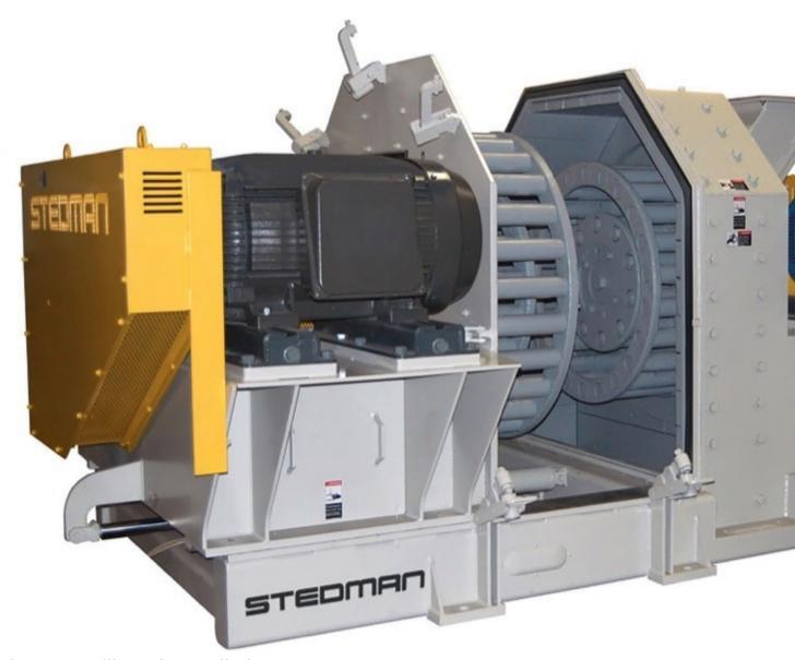
The cage mill can be applied to effectively crush, grind and pulverize a broad array of abrasive and non-abrasive materials, including wet sticky types. (Pictures: ©Stedman Machine Company)
