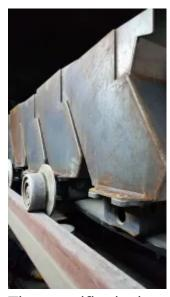
The specific design of the BEUMER system's cell strand facilitates the clean transportation of the clinker – no clinker can run out.
